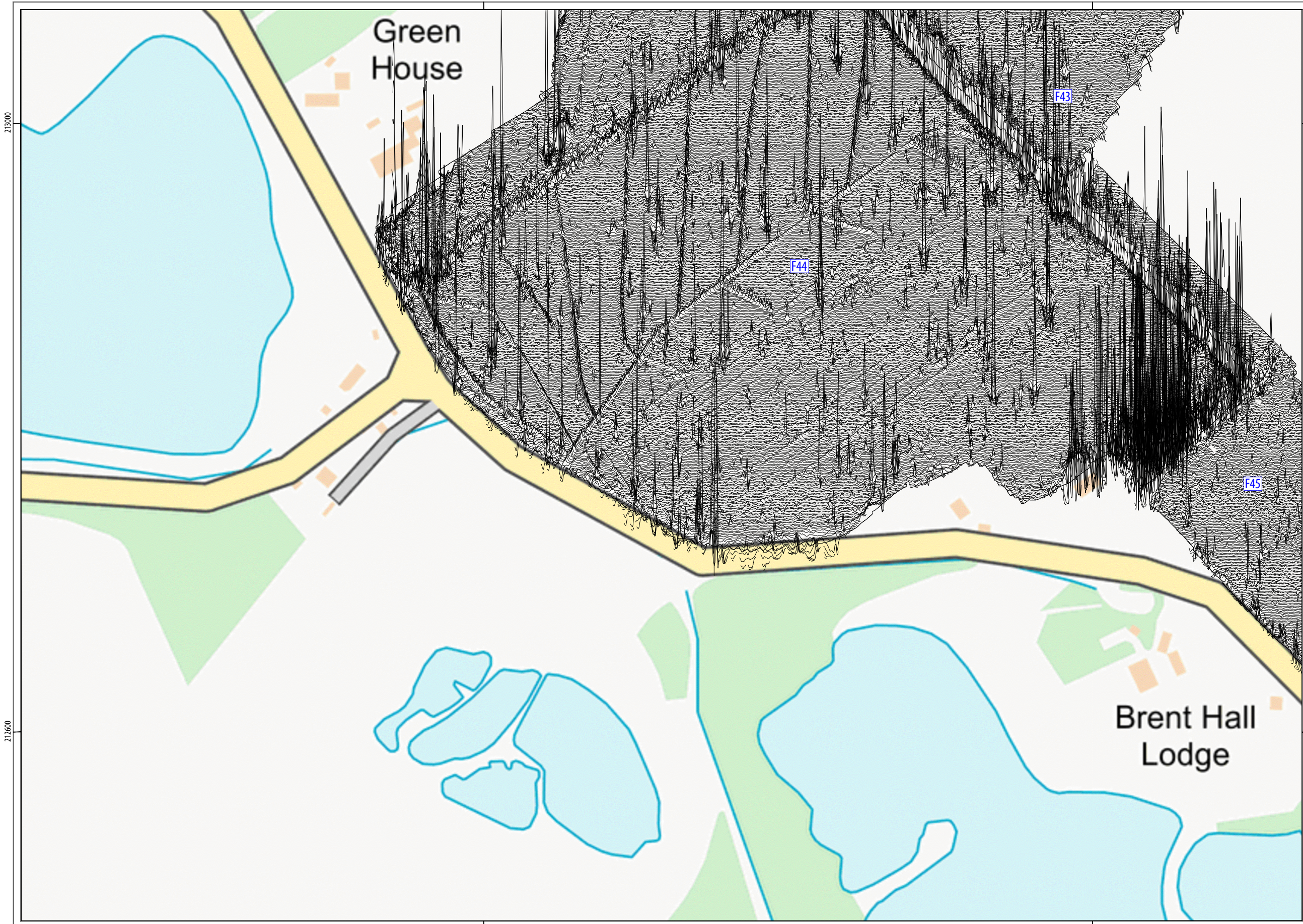
ILLUS 59 XY trace plot of minimally processed magnetometer data; Area 16
