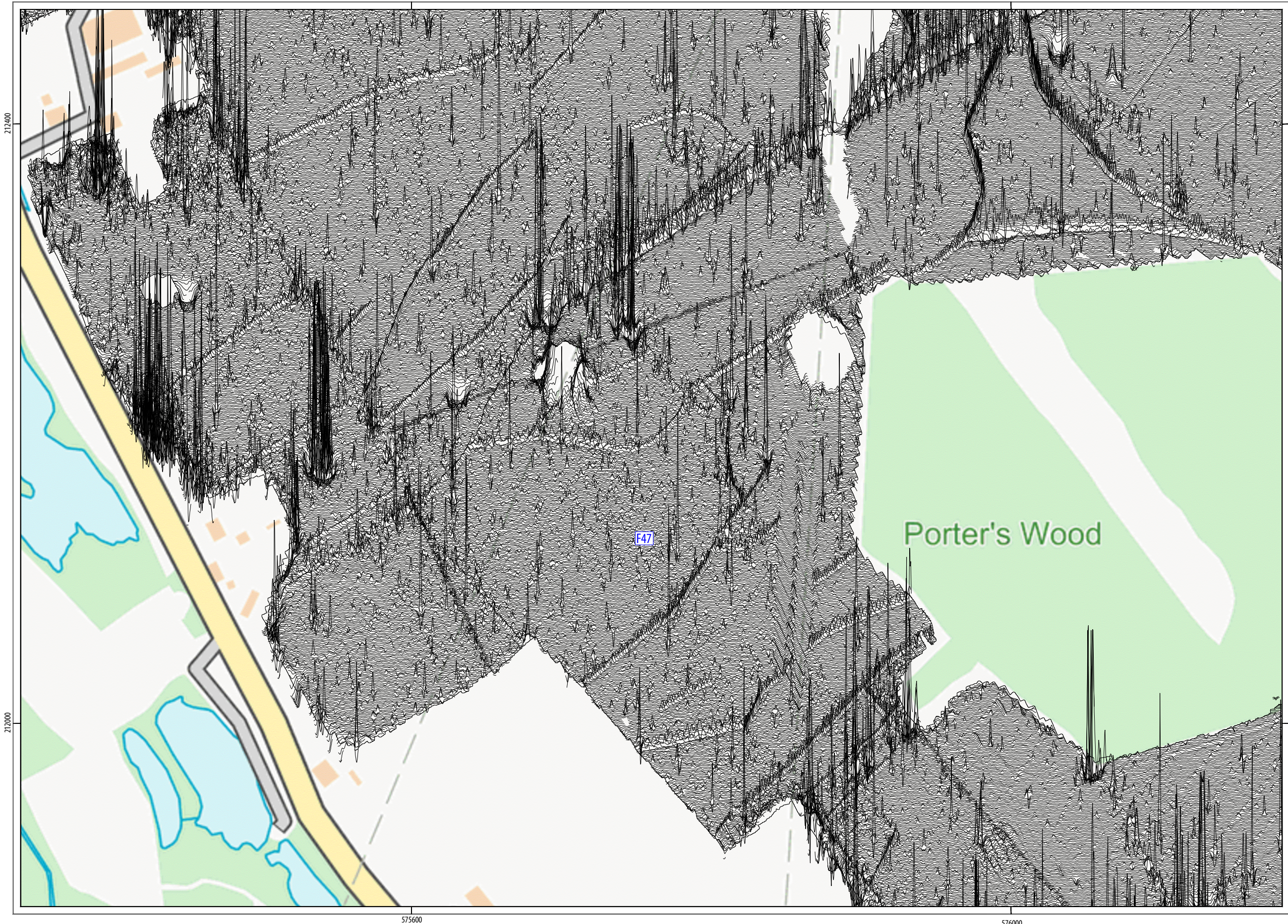
ILLUS 68 XY trace plot of minimally processed magnetometer data; Area 19
